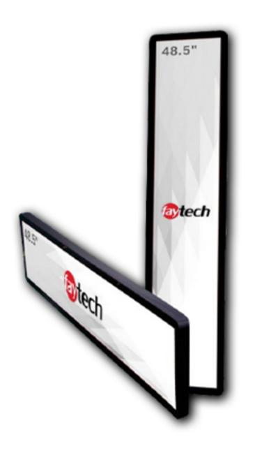
48.5" / 121.92 cm Screen diagonal Display active screen size 120.96 × 22.68 cm  $(47.62" \times 8.93")$ 48:9 Aspect ratio Physical resolution 1920 × 360 px Colours displayed 16.7M  $500 (cd/m^2)$ Brightness 4000:1 Contrast Typical reaction time Tr/Tf 8/8 (ms) Visual angle horizontal/vertical 178/178 (°) Backlight LED 30,000 (hours) Backlight lifetime
